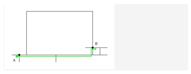
"Az  $XX^{\circ}$ " mark means Azimut it means the difference from North in degrees. In the example you should arrive to POINT B from a direction where you can leave that POINT to  $90^{\circ}$  from the North (it is East).
