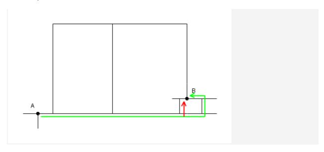
We don't have street in the real world as in the previous example. There is other street in the real world but based on the 5mm rule it is not a measurement error this should be handled as a street which is not marked on the map.
